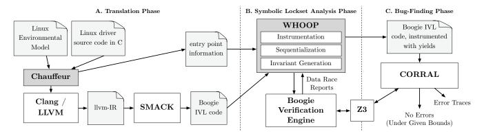
Fig. 7. The WHOOP architecture, empowered by state-of-the-art compilation (Clang/LLVM and SMACK) and verification (Boogie and CORRAL) tools.
