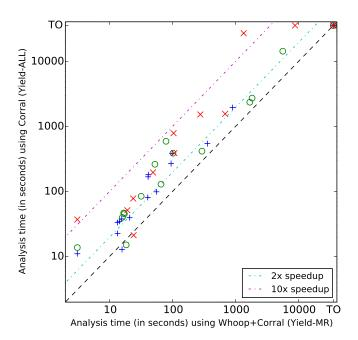
Fig. 9. Scatter plot showing the runtime speedups that CORRAL achieves using WHOOP with the Yield-MR instrumentation. The symbols +,  $\circ$ , and  $\times$  represent a context-switch bound of 2, 5, and 9, respectively.
