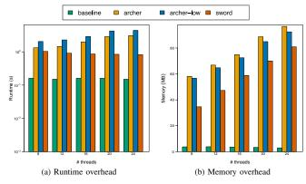
Figure 6: Geometric mean of runtime and memory overhead for OmpSCR suite; the number of threads varies from 8 to 24.
