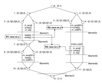
Figure 2: Structure of an OpenMP program, where  $m\_acq/m\_rel$  denotes a mutex acquire/release, IBarrier(id) an implicit, and Barrier(id) an explicit OpenMP barrier.
